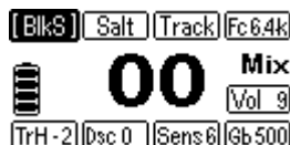
Fig. 2: Black Sand mode is activated
