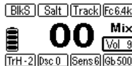
Fig. 16: Disc Mode is active
