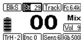
Fig. 4: Salt mode is activated and the salinity level is set to 29
