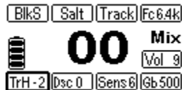
Fig. 7: Threshold is highlighted and can now be adjusted.
