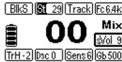
Fig. 14: Secondary Volume is highlighted and can be adjusted
