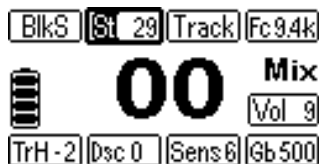
Fig. 4: Salt mode is activated and the salinity level is set to 29
